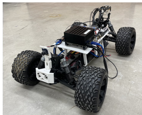
Figure 2: V-1 vehicle equipped with camera and MTi-7 sensor, LiDAR mount not pictured.
