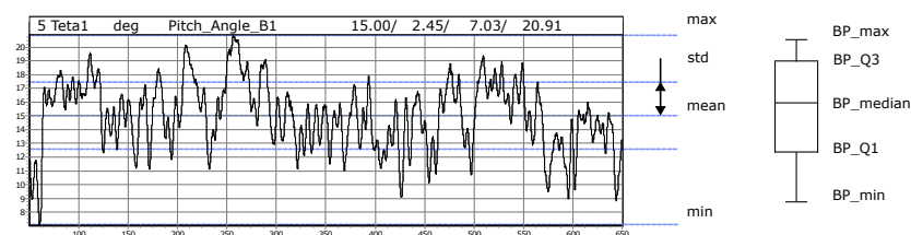
Figure 1: Representation of the outputs from the simulation and which features are taken from the time series.
