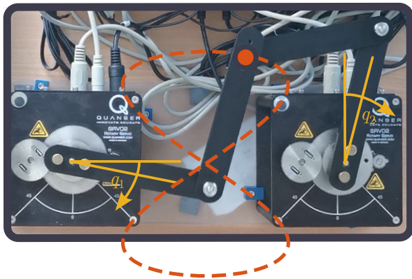
Figure 1: The identified five-bar linkage mechanism. Coordinates q_1, q_2 represent the controlled joints' rotation.
