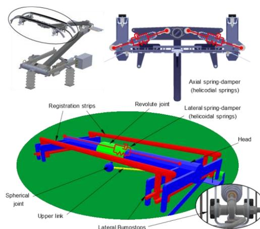
Figure 1: HSX MB pantograph model
