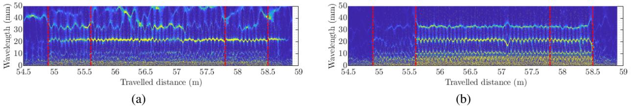
Figure 3: The time frequency analysis of the ABA measurements by using Wavelet Synchrosqueezed Transform (WST). (a) Longitudinal direction (b) Vertical direction.
