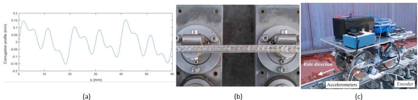
Figure 1: (a) Profile of designed corrugation, (b) Real corrugation in scaled track, (c) Scaled vehicle.
