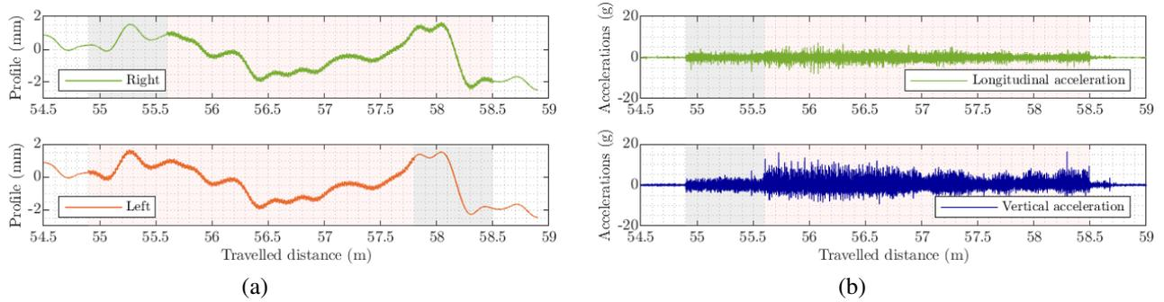
Figure 2: (a) Vertical profiles at left and right rails, (b) The ABA measurement on the right axle-box with forward velocity  $V = 0.5$  m/s in vertical and longitudinal directions
