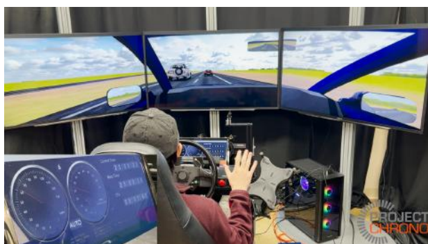
Figure 3: Chrono::HIL used for studying human-automation interplay.
