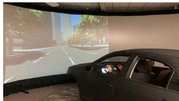
Figure 2: Chrono::HIL coupled with full-cabin simulator.
