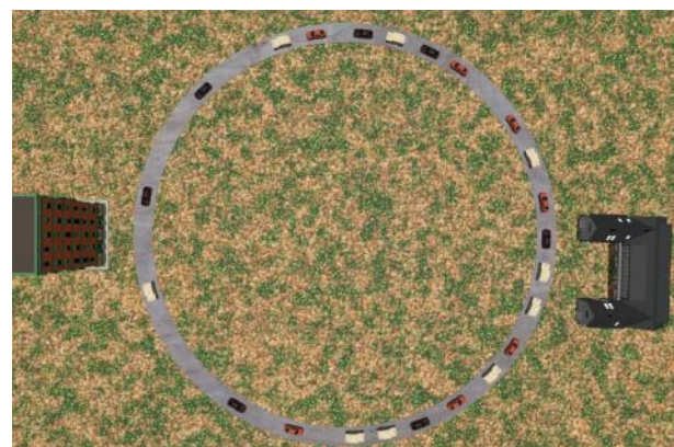
Figure 4: A ring experiment to explore traffic pattern using Chrono::HIL. The simulation involves 23 vehicles, including 1 human-driven vehicle and 22 autonomous vehicles.
