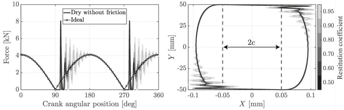
**Figure 5.** Restitution coefficient  $c_r$  sensitivity: normal contact force (left); pin center trajectory (right).
