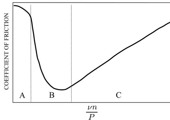
**Figure 1.** Stribeck curve: friction coefficient varying the ratio between the product viscosity times rotational speed ( $\nu n$ ) and the load ( $P$ ) .
