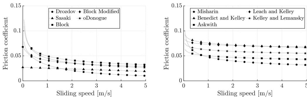
**Figure 2.** Friction coefficient varying sliding speed for different semi-empirical formulations.
