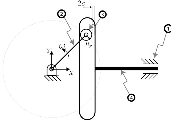
Figure 3. Scotch-Yoke mechanism with pin-slot non-ideal joint.
