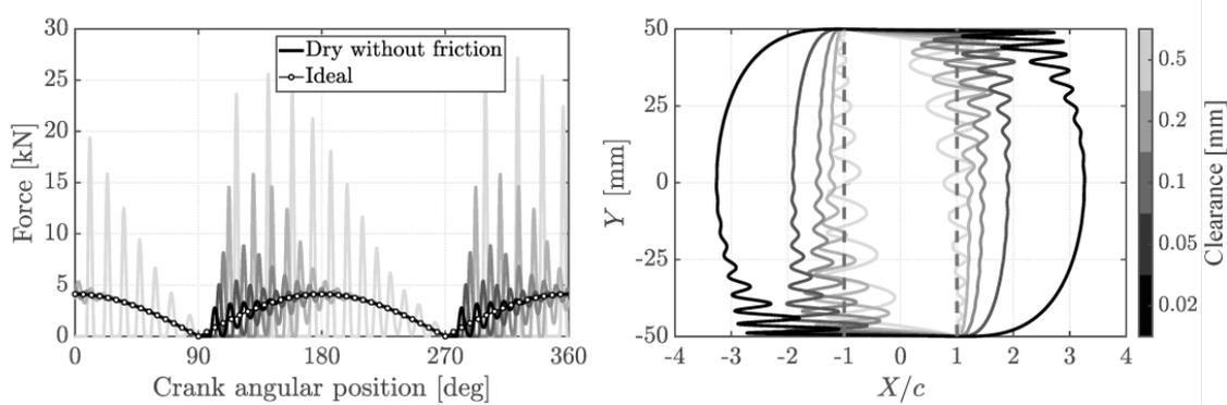
**Figure 4.** Clearance  $c$  sensitivity: normal contact force (left); pin center trajectory (right).
