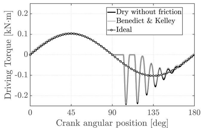
**Figure 9.** Comparison of driving torque between ideal and non-ideal cases.
