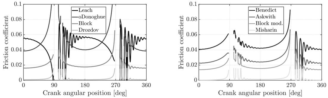
**Figure 7.** Friction coefficient for different semi-empirical formulations.
