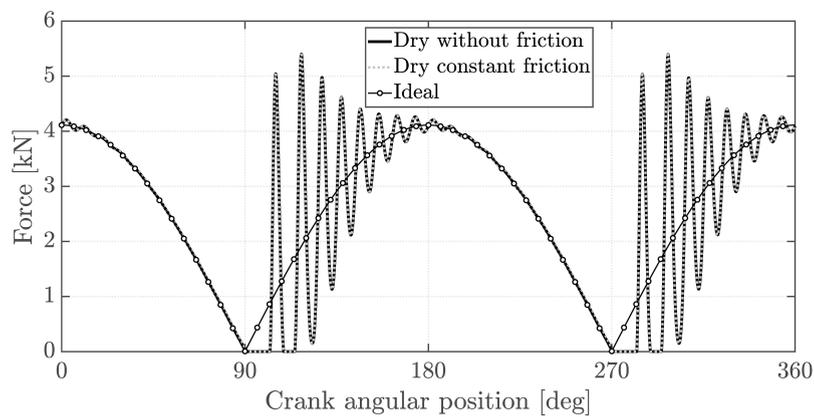
**Figure 6.** Comparison of normal contact force in non-ideal joint with reaction force of ideal joint.
