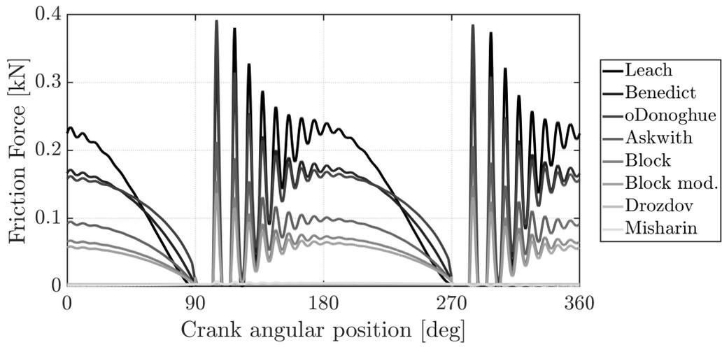
**Figure 8.** Friction force for different semi-empirical formulations.
