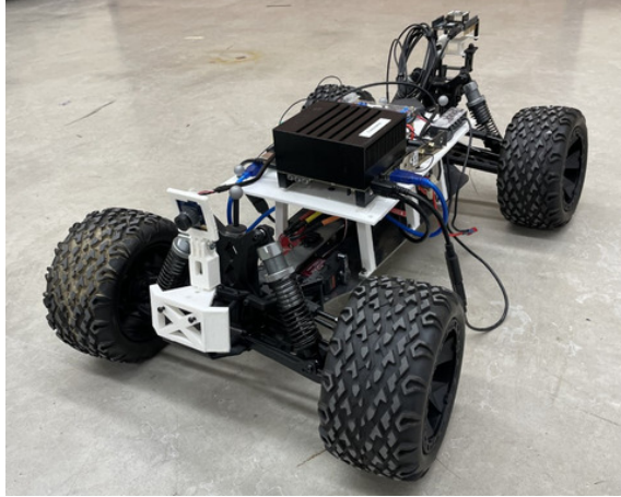
Figure 1: 1/6th scale autonomous vehicle (V-1) showing 3D printed reconfigurable mountings and support of camera, imu/gnss, and Jetson AGX, the later running the autonomy stack.
