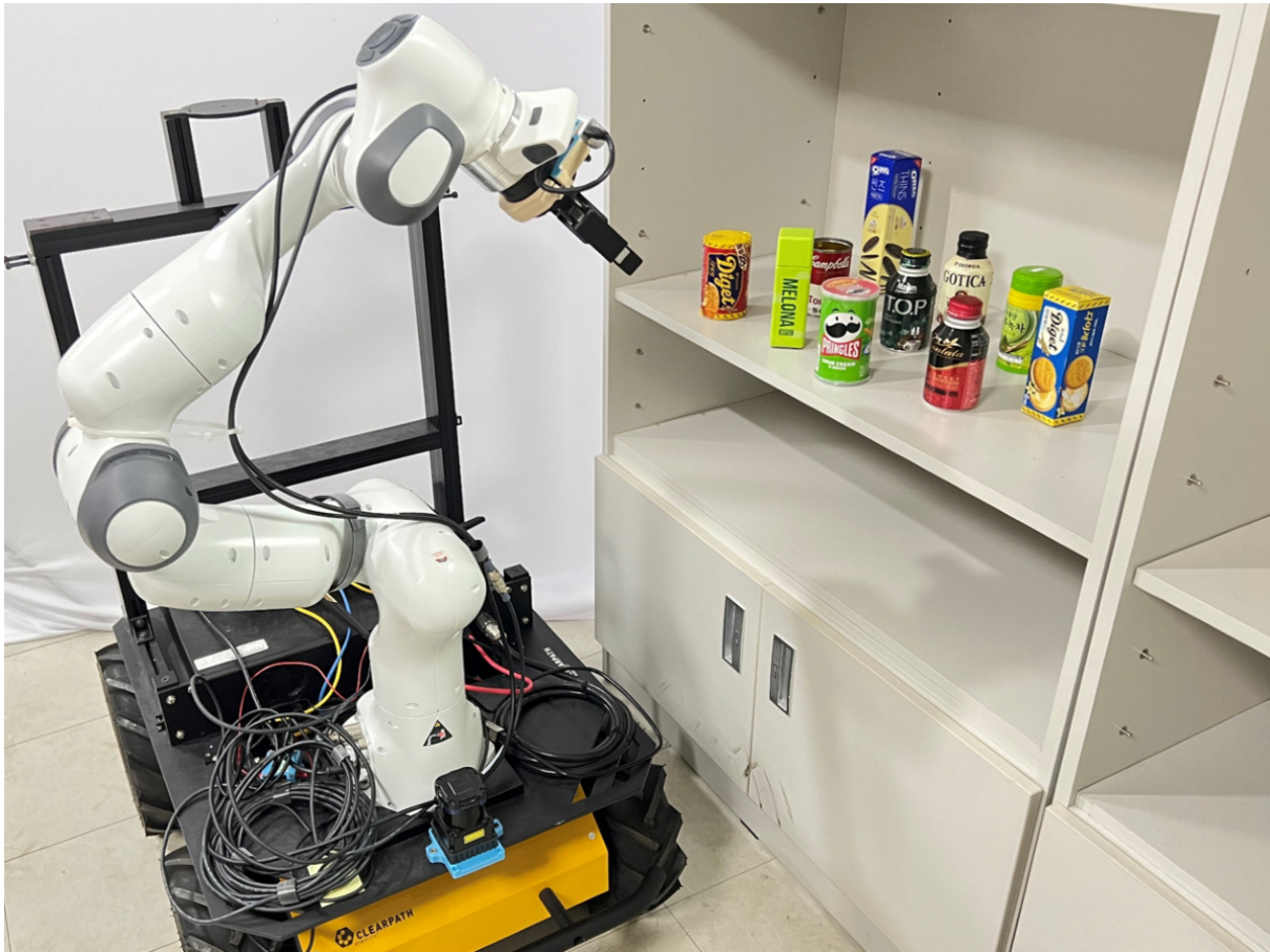
Fig. 1: An example of cluttered environment. Various objects are placed on the shelf. Some objects need to be removed to grasp a target object without collisions against the other objects and the boards.
