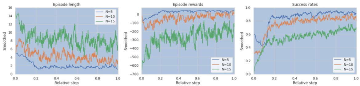
Fig. 5: The results of learning for the OR-TAMP problem. The x-axis of each graph represents a relative step. The models with N=5 , N=10 and N=15 stop learning at 40K, 60K and 100K steps, respectively.
