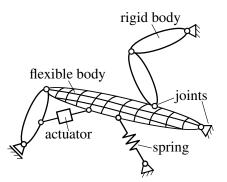
Figure 1: Schematic flexible multibody system
