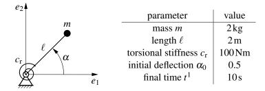
Figure 2: Application example torsional spring pendulum
