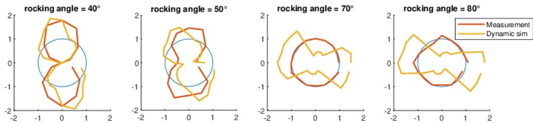
**Figure 8.** Layer thickness distribution at a rocking angle (RA) of 40, 50, 70 and 80 degrees
