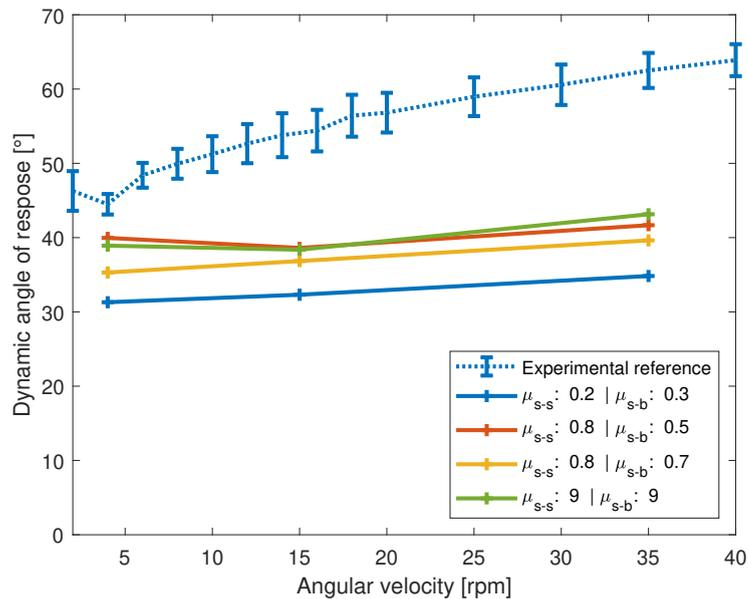
**Figure 6.** Dynamic angle of response when altering the sphere-sphere friction coefficient
