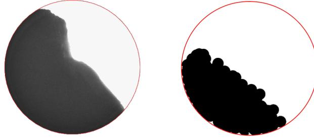
**Figure 3.** Exported image from the Granutools GranuDrum setup (left) and the DEM-simulation (right)
