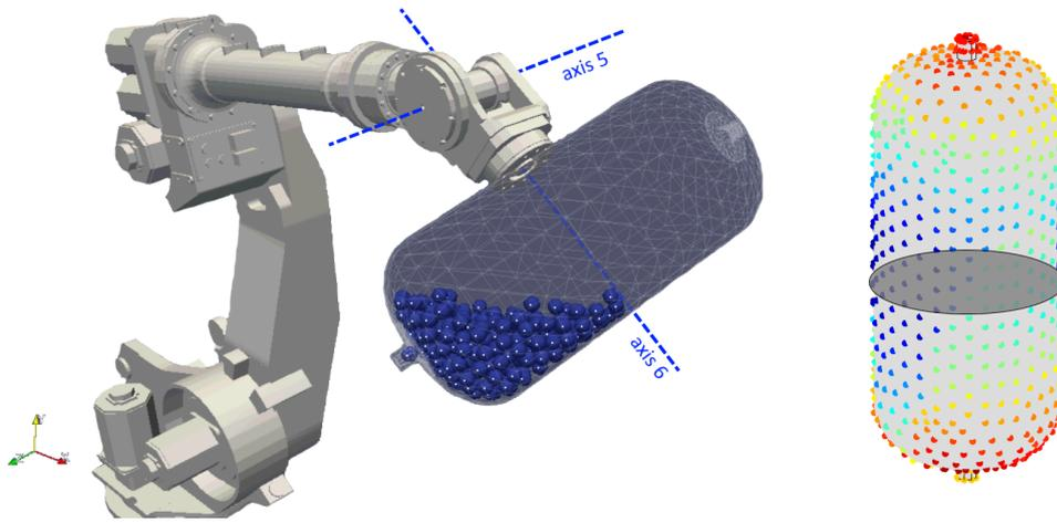
**Figure 4.** Robomould MBD-DEM co-simulation (left) and the measurement points (right)
