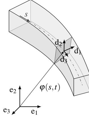
Figure 2: Sketch of the geometrically exact beam
