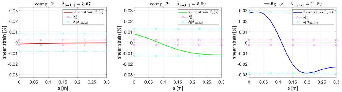
**Figure 5.** Simulated shear strain (*left*: config. 1, *middle*: config. 2, *right*: config. 3), together with rough estimate  $\lambda_0^2$  and improved estimate  $\lambda_0^2 \bar{\lambda}_{[m,f,r]}$ .
