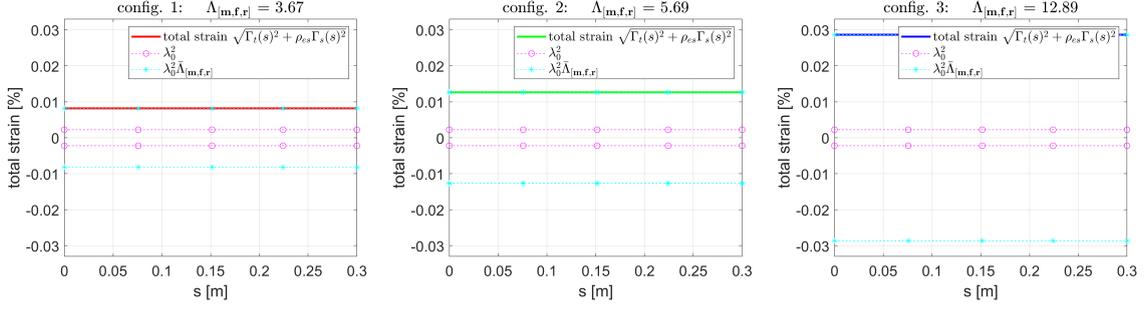
**Figure 6.** Simulated total extensional & shear strain values (*left*: config. 1, *middle*: config. 2, *right*: config. 3), together with rough estimate  $\lambda_0^2$  and improved estimate  $\lambda_0^2 \bar{\Lambda}_{[m,f,r]}$ .
