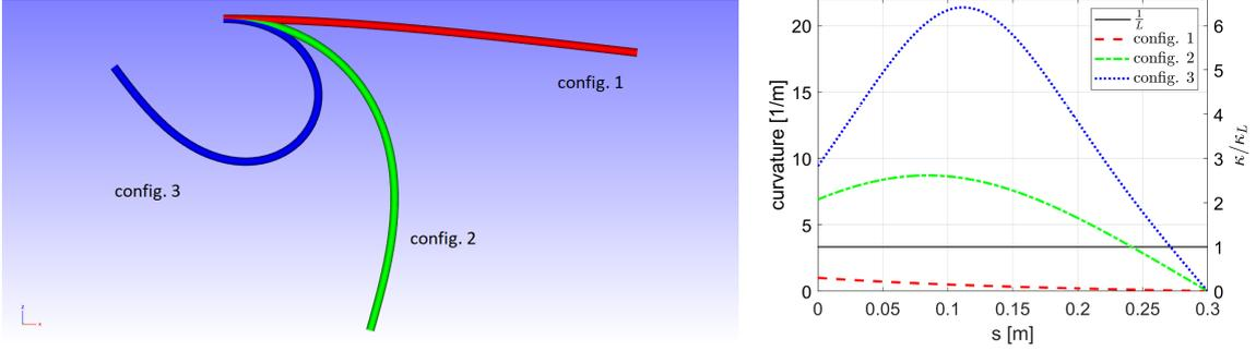
**Figure 3.** *Left:* Three different example configurations, all with plane bending. *Right:* Curvature along the rod with two different y-axes (in [1/m] and dimensionless in units of  $\kappa_L$ ). Numerical solutions are computed by minimization of the elastic energy subject to the prescribed boundary conditions (see [5] for details).
