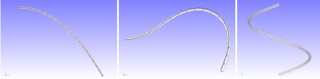
**Figure 2.** Analytical centerline curves of an inextensible Kirchhoff rod (solid lines) in plane bending (*left*: cantilever type, *middle*: both ends clamped) and helical (*right*) configurations. The red dots show the vertex positions computed with a discrete Cosserat rod model by minimization of the elastic energy (see [5] for details).
