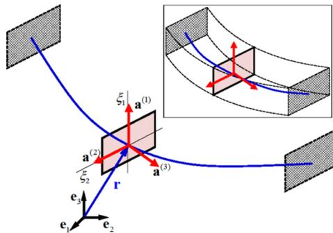
**Figure 1.** Centerline  $\mathbf{r}(s)$  and moving frame  $\mathbf{R}(s) = \mathbf{a}^{(k)}(s) \otimes \mathbf{e}_k$  of a Cosserat rod (see [3]).
