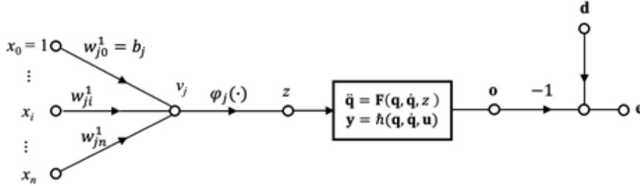
Figure 3. One signal-flow graph representation of neuron  $j$  in contact with physical model.
