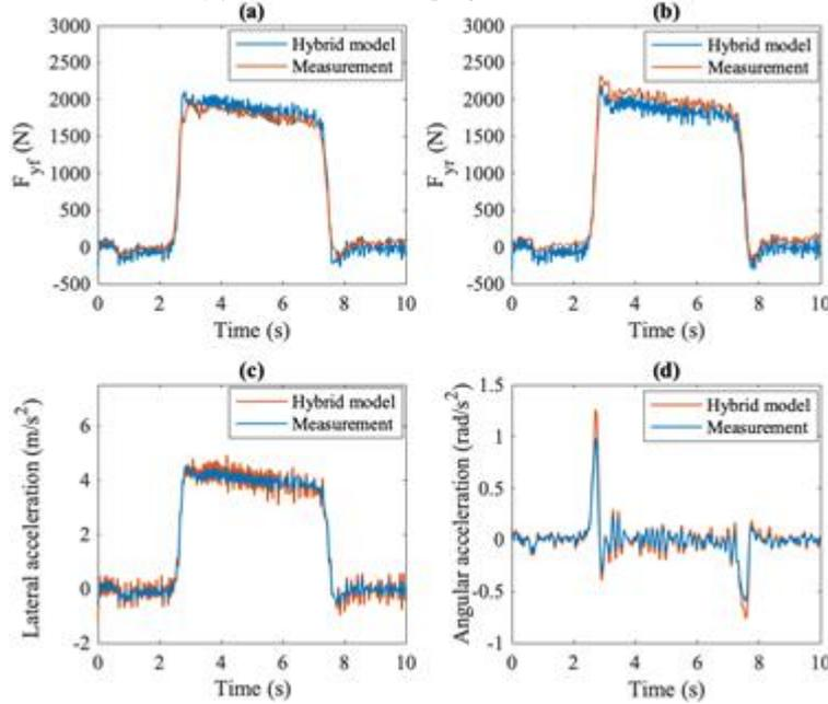
**Figure 7.** Estimating lateral forces from step maneuver data: (a) front wheel lateral forces, (b) rear wheel lateral forces; (c) lateral acceleration; (d) angular yaw acceleration.
