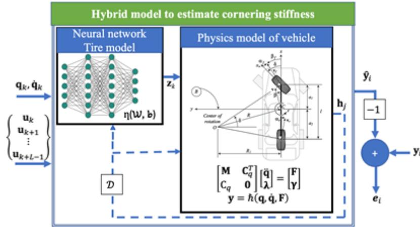
**Figure 2.** Hybrid model to estimate lateral forces,  $\mathbf{z}_k: \{C\alpha_f, C\alpha_r\}$  or  $\{F_{yf}, F_{yr}\}$ ,  $j: k+1 \rightarrow k+L$ ,  $\mathbf{y}_i = [y_k \quad y_{k+1} \quad \dots \quad y_{k+L-1}]$ ,  $\hat{\mathbf{y}}_i = [\hat{y}_k \quad \hat{y}_{k+1} \quad \dots \quad \hat{y}_{k+L-1}]$ .
