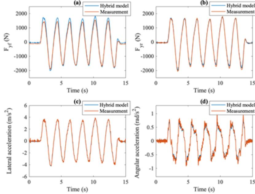
**Figure 8.** Prediction of lateral forces from sine maneuver data: (a) front wheel lateral forces, (b) rear wheel lateral forces; (c) lateral acceleration; (d) angular yaw acceleration.
