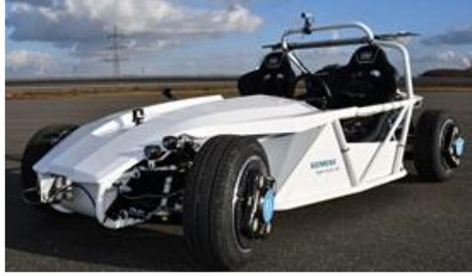
**Figure 4.** Siemens SimRod electric vehicle, equipped with wheel force transducers.
