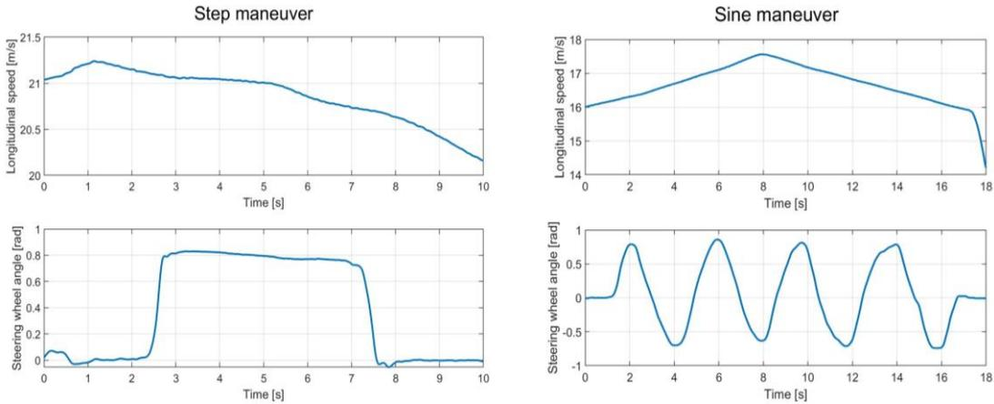
**Figure 5.** Profiles of longitudinal speed and steering wheel angle for step and sine maneuvers.
