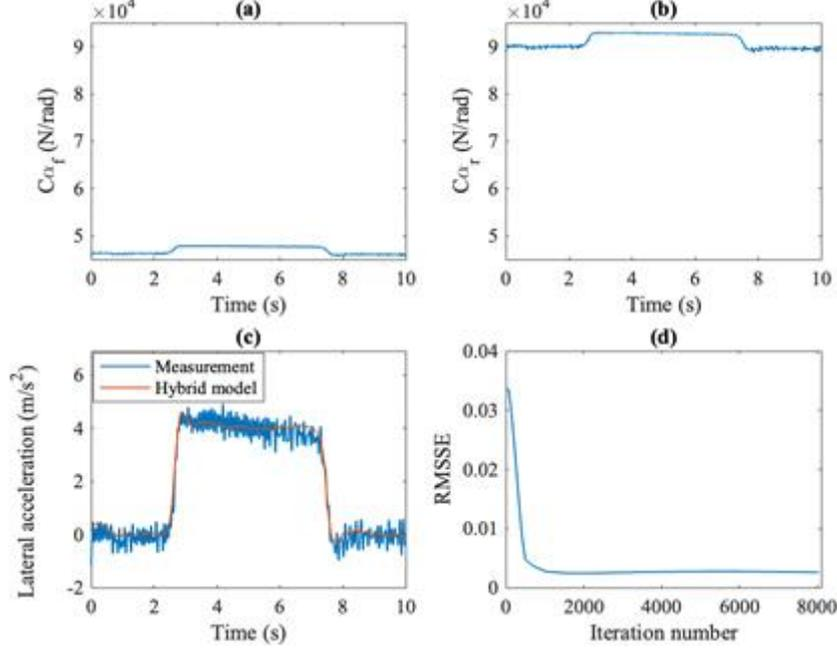
**Figure 6.** Estimating cornering stiffness: (a) front wheel cornering stiffness, (b) rear wheel cornering stiffness; (c) lateral acceleration; (d) root mean sum of squared error.
