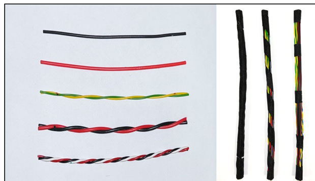
Figure 1. Examples of different types of cables, unshielded twisted pairs and triples (from top to bottom on the left) and cable bundle specimens with different taping patterns (right).
