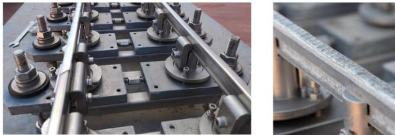
**Figure 16.** Corrugation in the scale track.
