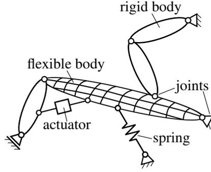
Figure 1: Schematic flexible multibody system
