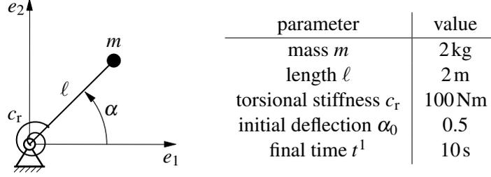
Figure 2: Application example torsional spring pendulum
