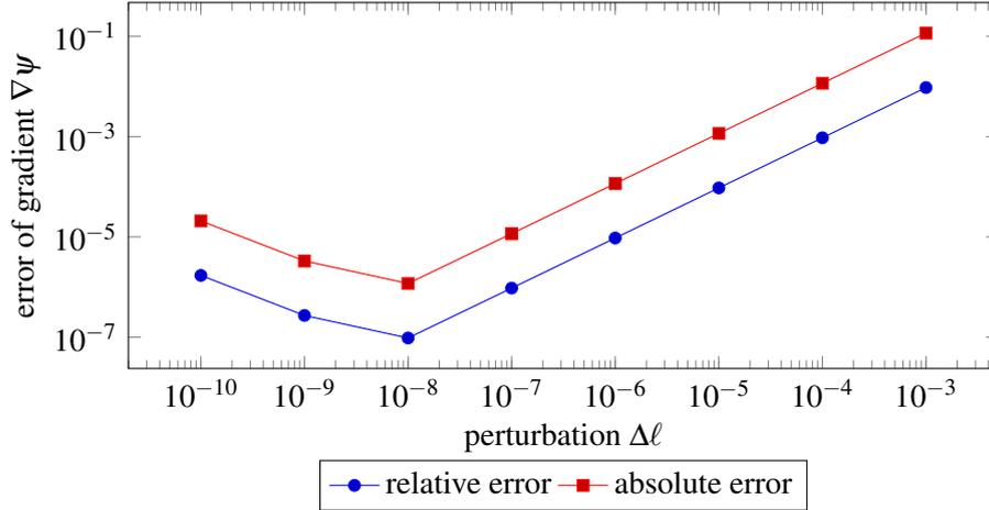
Figure 4: Gradient error using the finite difference method
